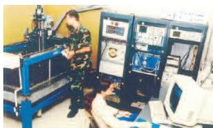
**Figure 6. A Materials Engineer Positions the Ultrasonic Transducer for a Scan while a Computer Specialist Enhances Scanning and Image Analysis Capabilities.**
