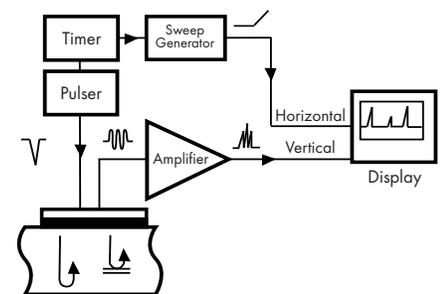
**Figure 1. Basic Pulse Echo System for Ultrasonic Testing. [5]**
