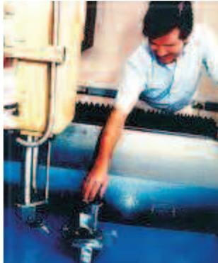
**Figure 4. A Prototype Composite Airfoil is Aligned for Ultrasonic Inspection. Automated inspections can be made of small or large components in this tank.**
