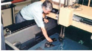
**Figure 3. An Impact-Damaged Graphite/Epoxy Specimen is Positioned for Inspection in the Immersion Tank for Large Structures.**
