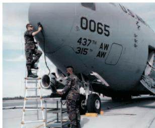
**Figure 5. Manual Ultrasonic Inspection of an Aircraft.**
