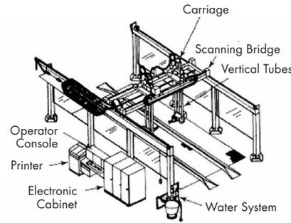
**Figure 2. Large Automated Quality Control System Containing Modular Ultrasonic Test Component.[5] (Copyright 2007 © Reprinted with permission from the American Society for Nondestructive Testing.)**
