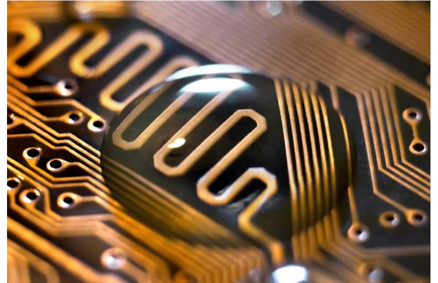
High-speed signals are often length matched.
