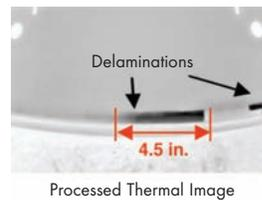
**Figure 3. Delaminations on Shuttle leading edge discovered using thermography.**
