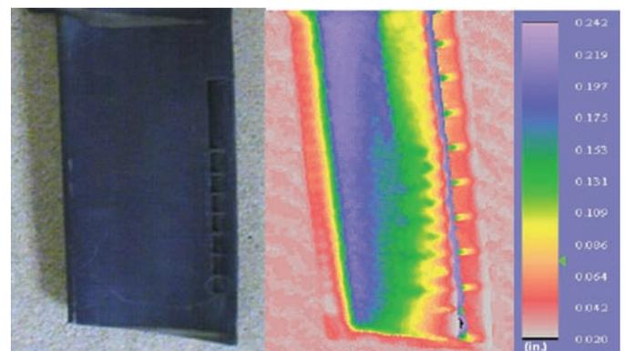
**Figure 5. Thermograph of power turbine blade showing wall thickness. (Photo Courtesy of Thermal Wave Inc.)**
