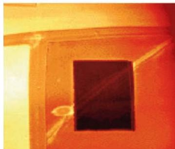
**Figure 6. Thermal inspection of E2-C Hawkeye propeller. [8]**
