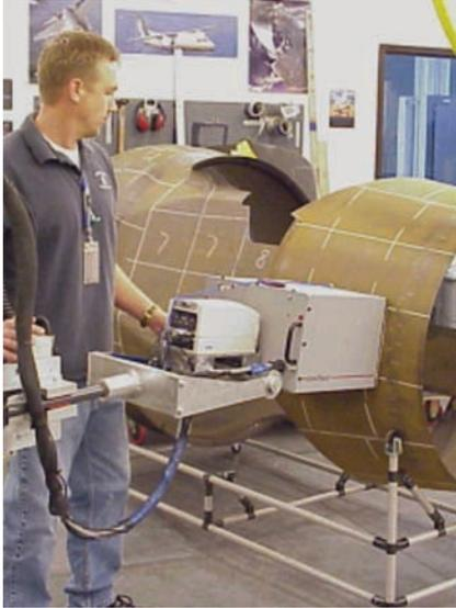
**Figure 4. Thermographic evaluation by mapping local sample points using TSR. [6]**
