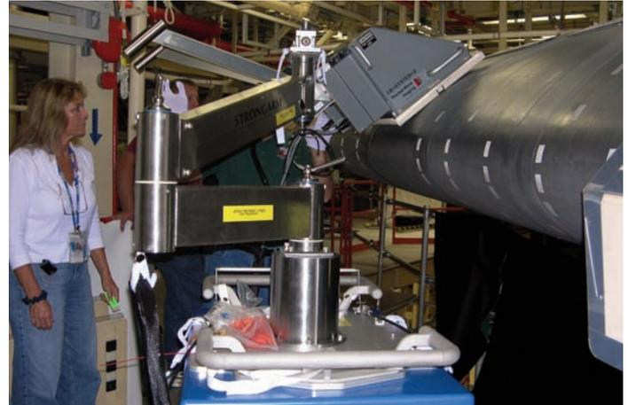
**Figure 2. Thermographic inspection of Space Shuttle leading edge. [7]**
