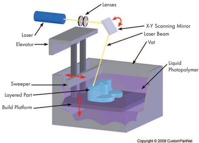
**Figure 1. An illustration of the stereolithography process. (Image courtesy of CustomPartNet, Copyright © 2008)[12]**
