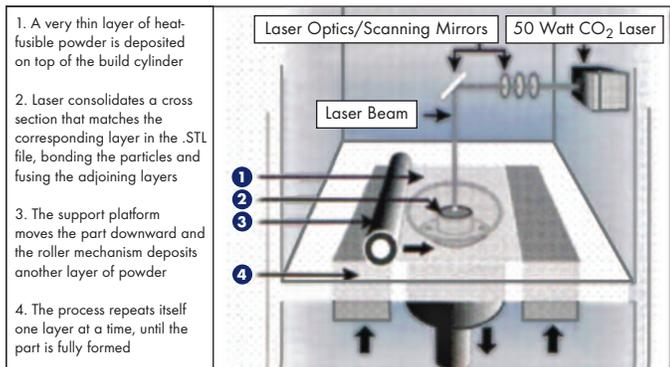
**Figure 2. Selective laser sintering process.[3]**
