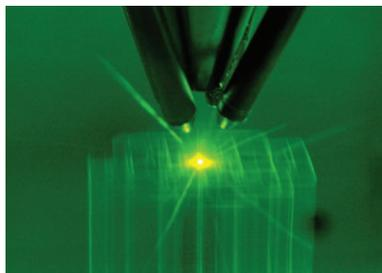
**Figure 1. Four nozzles deliver powder sintered by a laser beam into a Sandia thunderbird logo design. (Photo by Randy Montoya and provided courtesy of Sandia)**
