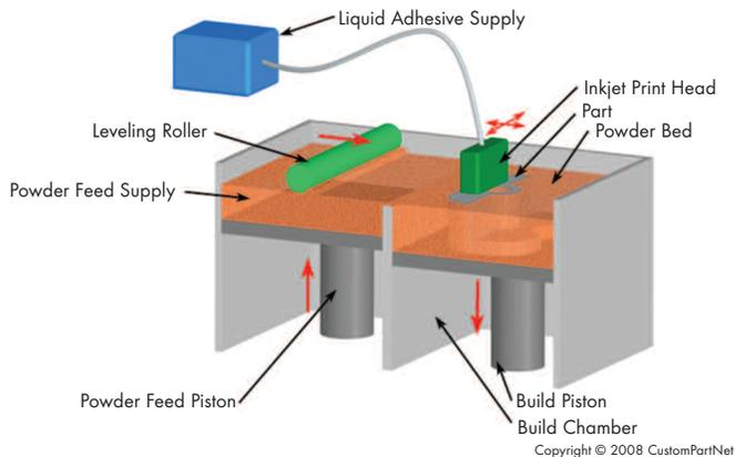
**Figure 3. Three-dimensional printing process. (Image courtesy of CustomPartNet, Copyright © 2008)[31]**
