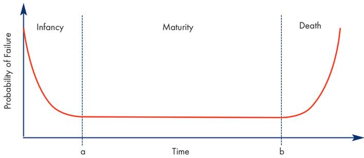
**Figure 3. Bath tub curve.**
