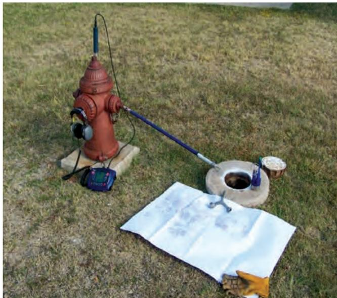
**Figure 3. Acoustic emissions testing being used to monitor a fire hydrant for leaks. (Photo courtesy of U.S. Army Corps of Engineers.)**[16]
