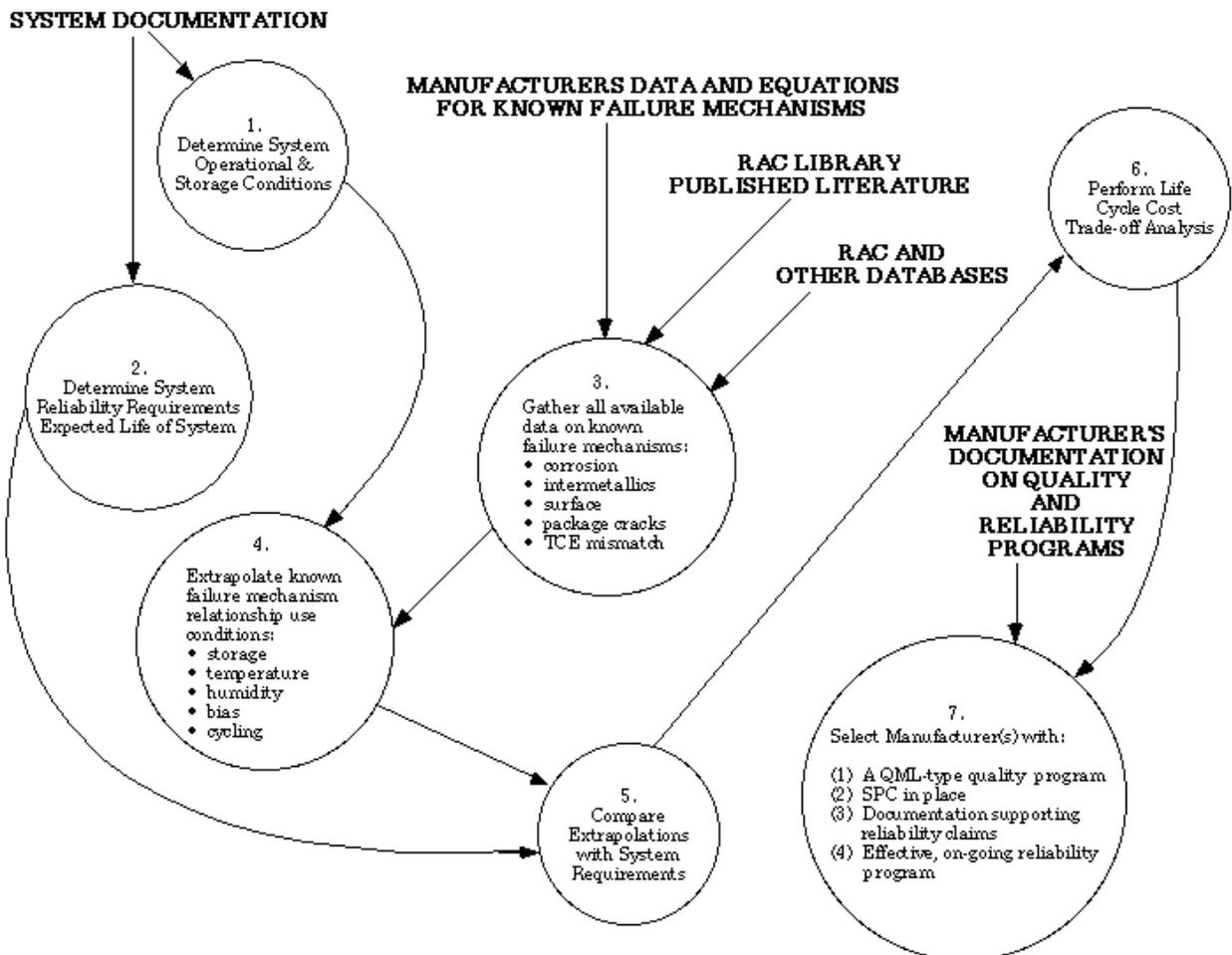
Figure 2: Process Flow for PEM Use Determination
