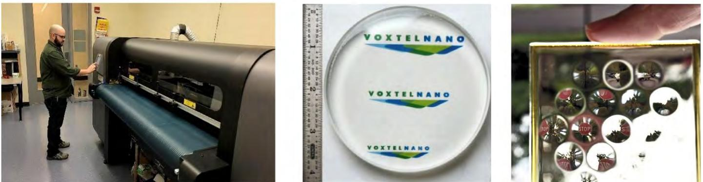
Figure 3: Voxel’s Medium-Scale VIRGO AM Platform (Left), 4-inch-Diameter GRIN Lens and Phase Corrector Plate (Center), and Lenslet Arrays (Right) (Source: Voxel, Inc.).
