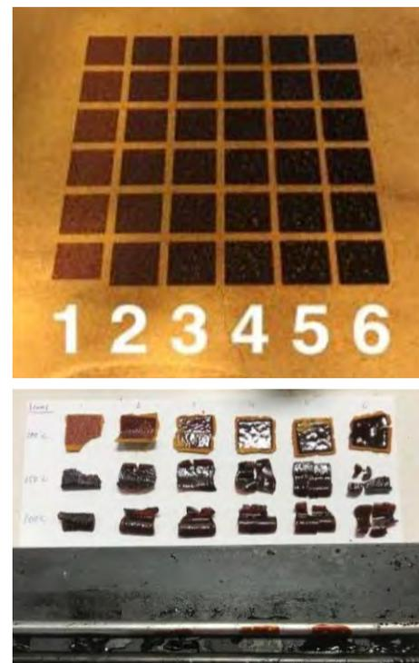
Figure 3: Puddle Formation During Postprocessing Neat Polyimide Resin After Laser Consolidation (Source: AFRL).
