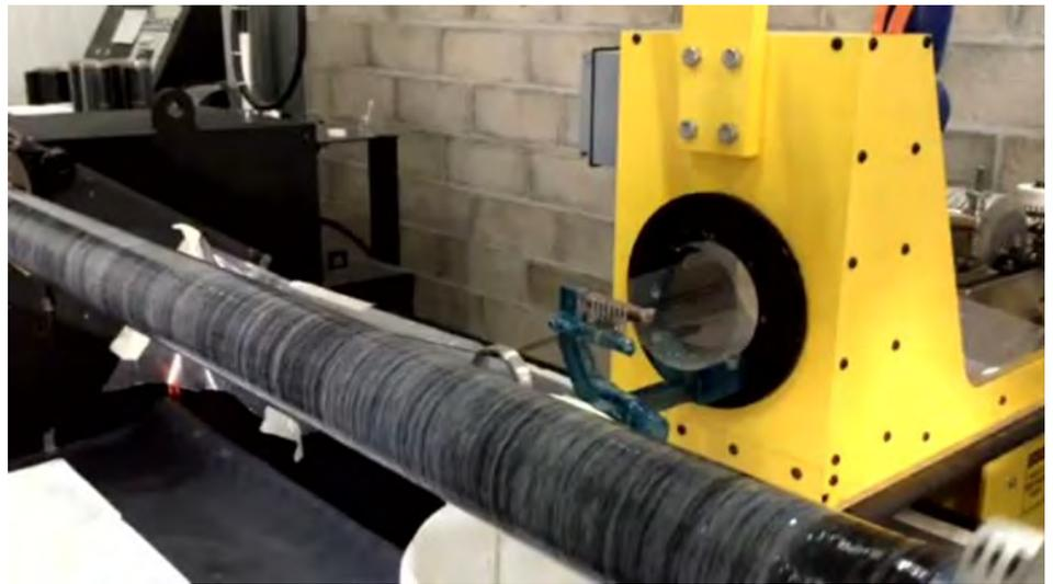
Figure 1: Winding the Composite Tube (Source: U.S. Army Combat Capabilities Development Command Armaments Center [CCDC AC]).
