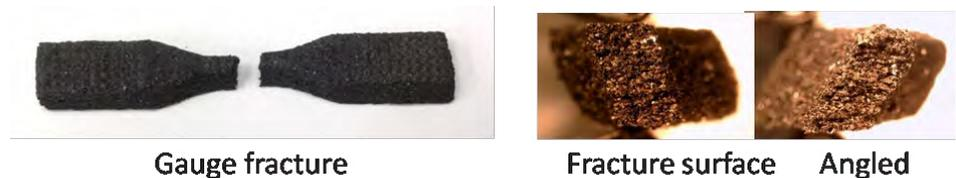
Figure 6: Images of a Fractured Specimen After Tensile Testing (Source: AFRL).
