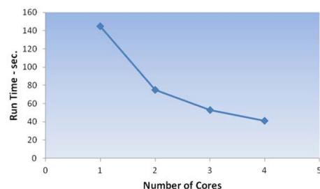
Figure 5. Simulation Results for Different Numbers of CPU Cores.
