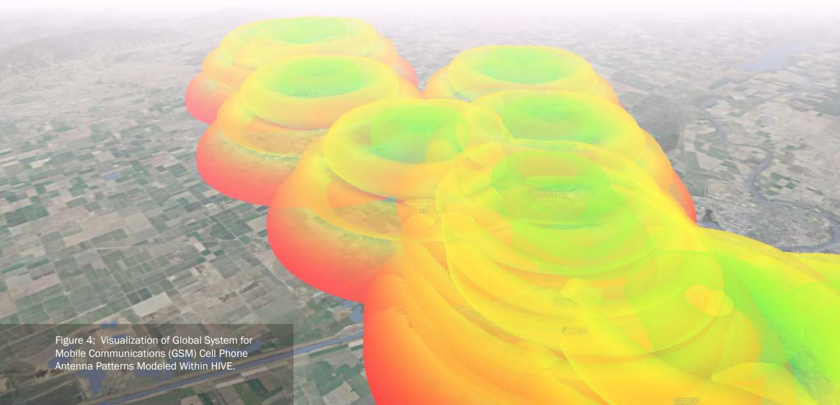
Figure 4: Visualization of Global System for Mobile Communications (GSM) Cell Phone Antenna Patterns Modeled Within HIVE.
