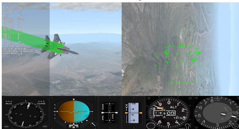
Figure 5: The Default BlueMax Cockpit in HIVE With Basic Flight Displays, a Heads-Up Display (HUD), and a Third-Person View of the Aircraft.
