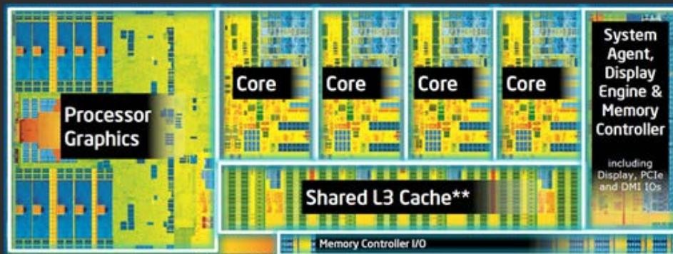
Figure 1: Typical Multi-Core CPU.
