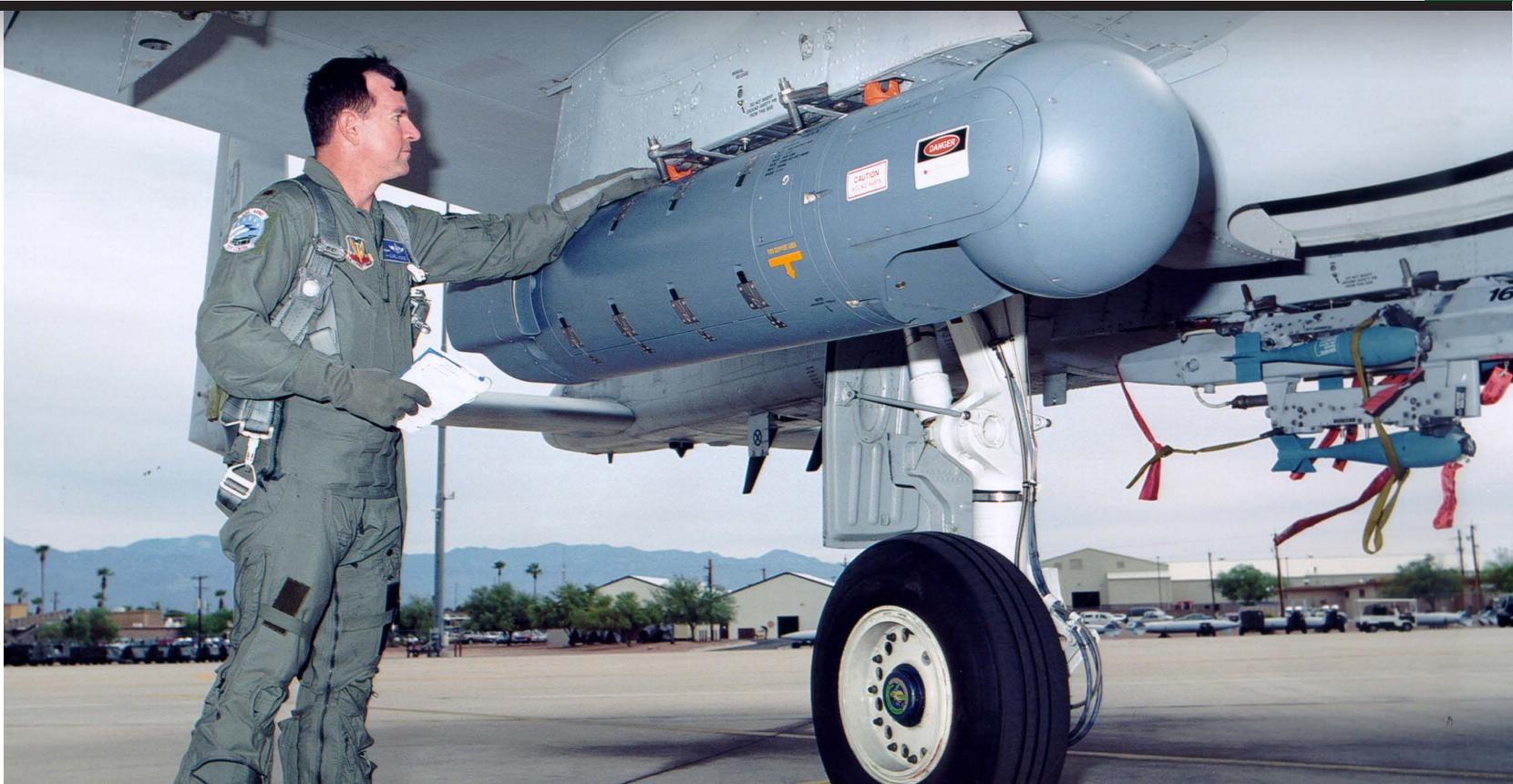
Figure 7: The USAF LITENING G4 LTIP Pod Using Active Imaging for Extended Range Target ID (Northrop Grumman).
