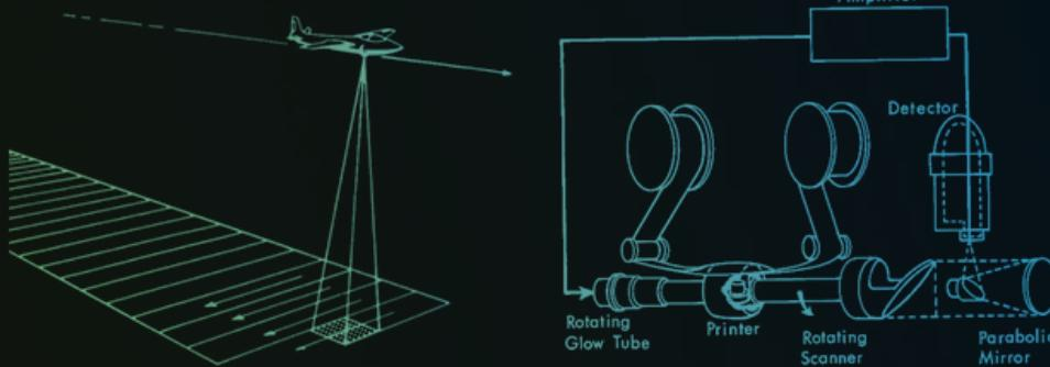
Figure 2: Illustration of an IR Mapper, Where an Image Scanned by a Rotating Mirror Is Transferred to Film via a Synchronously Scanning Glow Tube Modulated by the IR Detector Output. The Aircraft's Forward Motion Adds the Second Dimension to the Raster Scan [5, 6].
