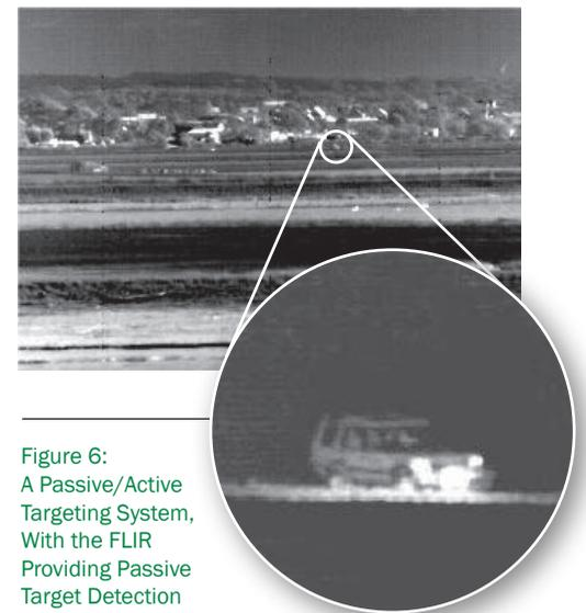
Figure 6: A Passive/Active Targeting System, With the FLIR Providing Passive Target Detection and the LADAR Providing Active Identification [12] (Copyright BAE, UK, All Rights Reserved).
