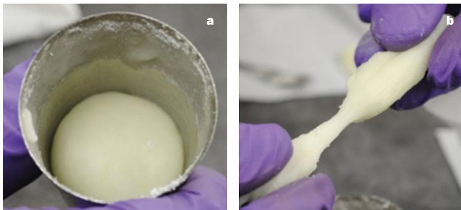
Figure 1: (a) RAM of AP Composite Propellant Feedstock Used and (b) Mix Consistency (Source: Naval Surface Warfare Center [NSWC]-IHEODTD).
