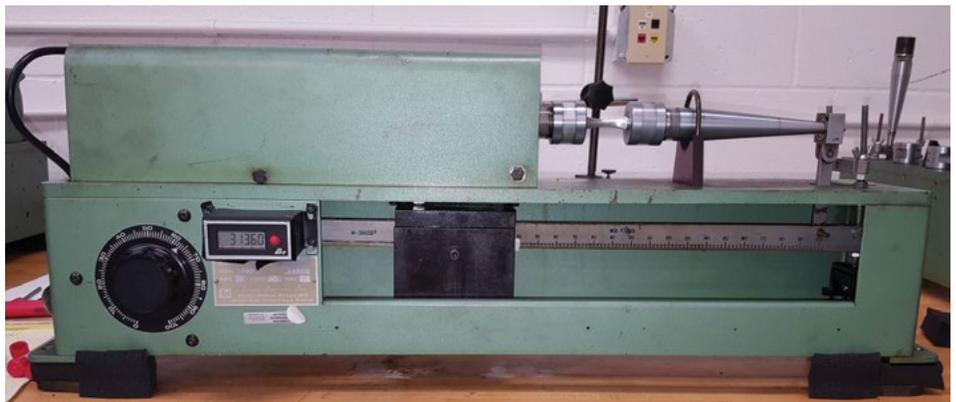
Figure 3: R.R. Moore Rotating Beam Test Apparatus With the Specimen Installed (Source: CCDC GVSC).
