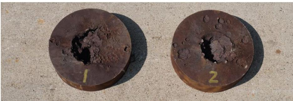
Figure 9: Steel witness plate penetration for Shot 1 (Left) and Shot 2 (Right) (Source: CCDC AC).
