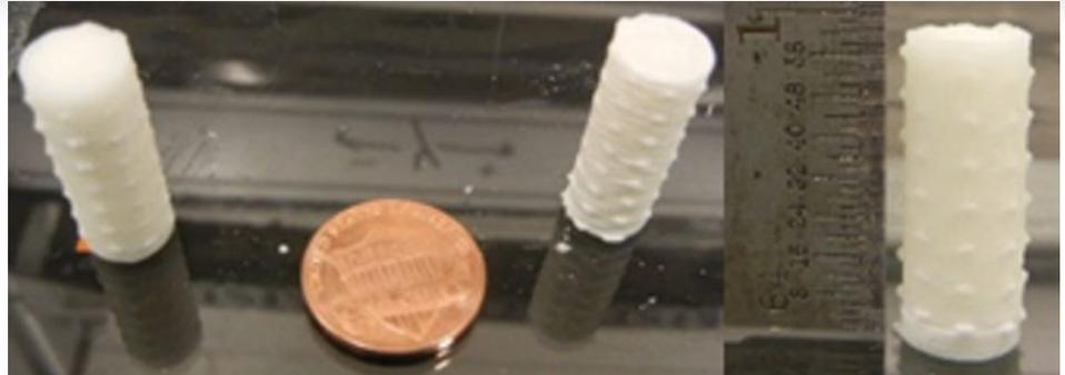
Figure 8: Repeated Grain Prints Utilizing Optimized Parameters With Retraction Time (Source: NSWC-IHEODTD).
