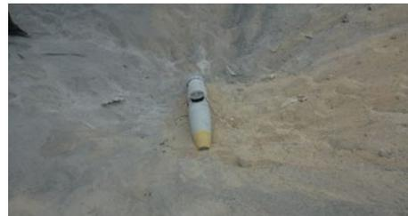
Figure 1: Placement of Cylindrical Dynamic Access Tool Prior to Initiation (Source: Sandia National Laboratories).
