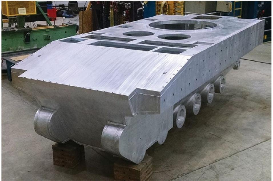
Figure 2: Friction Stir Welded Hull Prototype Designed by the Ground Vehicle Systems Center and Fabricated by Concurrent Technologies Corporation (Source: U.S. Army Combat Capabilities Development Command [CCDC] Ground Vehicle Systems Center [GVSC]).
