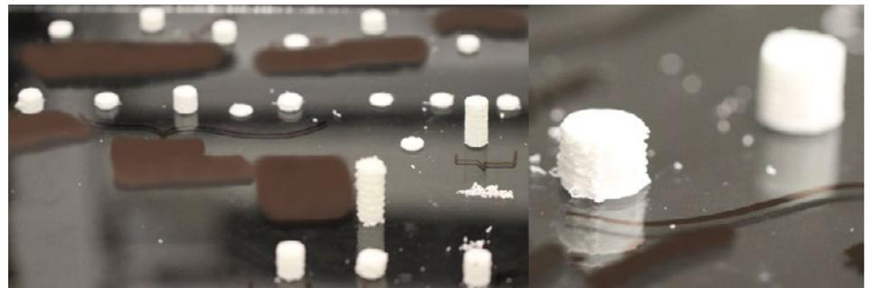
Figure 6: Failed Grain Prints Using Smaller Nozzle Sizes Due to Clogging (Source: NSWC-IHEODTD).
